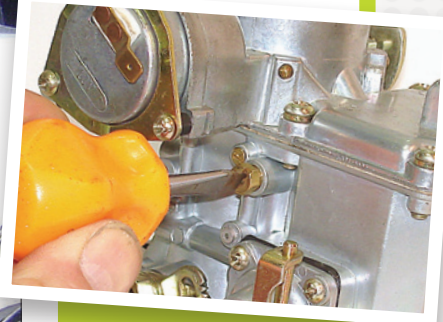
This picture shows the location of the idle jet in the carb, just above the accelerator pump diaphragm
