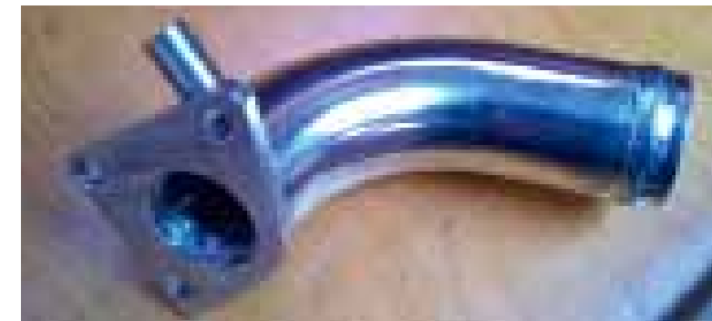
The new elbow was ordered online from the USA ( www.exhaustelbow.com ) and, including postage and customs, cost just less than half the price of the Yanmar part from a UK dealer. The new elbow, although not a Yanmar part, is made of stainless steel and looks and feels of very good quality
