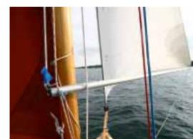
Instead of hooking to a ring on the mast, the inboard end of the pole remains attached to an uphaul/downhaul system.
