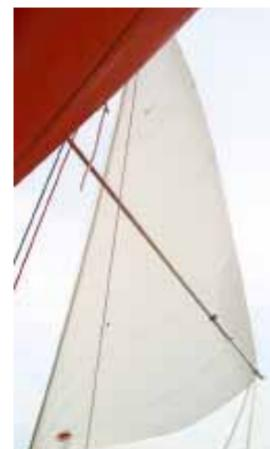
Here the pole's inboard end has been pulled down the mast to push the clew downwards and outboard, resulting in much more drive.
