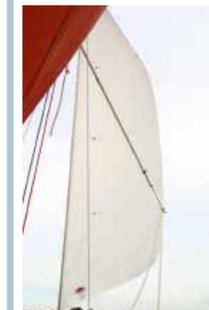
Despite being attached at both ends, the pole is doing nothing here: the jib is twisted open so far that much of the area is being wasted.
