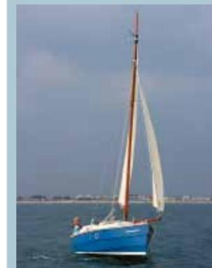
As the boat goes up a small wave, the yard swings inboard to create a mainsail with very little twist...
