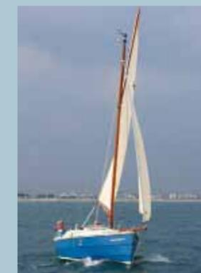
...but as the bow goes down to meet the next wave, the yard swings out and opens the leech.
