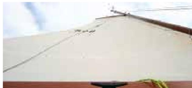
**CORRECT:** As the breeze picks up, or for sailing in flatter water, more outhaul tension creates a flatter sail.
