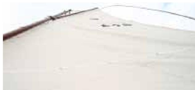
**WRONG:** The peak halyard needs to be eased downwind but, if it's not tensioned again for the beat, the result is this crease from throat to clew.
