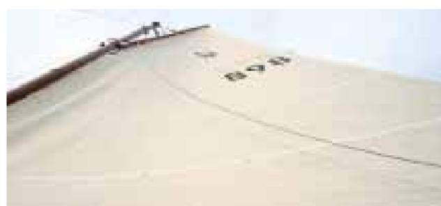
**WRONG:** Here the vertical crease means that the throat halyard, and therefore the luff, is too tight. If, on the other hand, it's hanging in bights between the lacing points, it's too loose.
