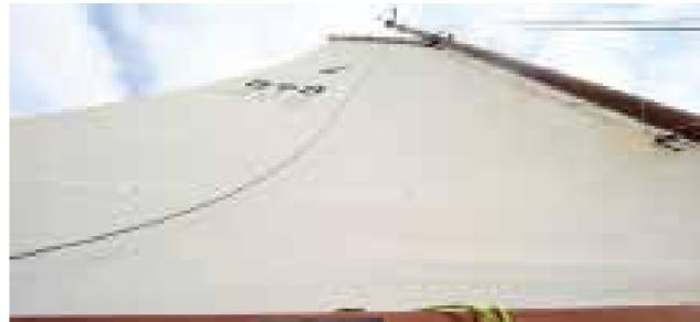
**CORRECT:** This is a good shape for upwind sailing when a full sail is needed, such as in light conditions in a seaway.
