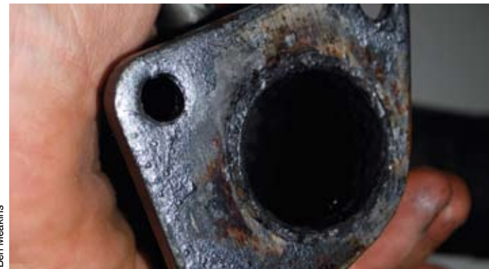
Polly's corroded exhaust elbow was not her only engine malady
