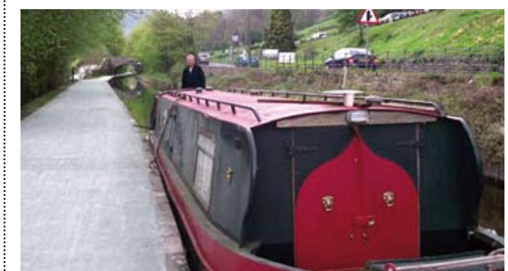
A flat bottom and 12.2m in front of the rudder precludes precise handling
