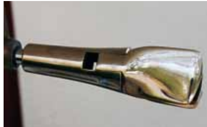
A mirror shine to the folding prop keeps fouling at bay for better speed
