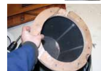
A ring of 25mm marine ply is attached to the rim of the bucket
