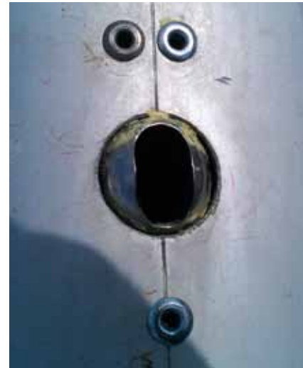
The cap shroud backing plates have hairline cracks at the edges of the socket – but their replacements are subtly different
