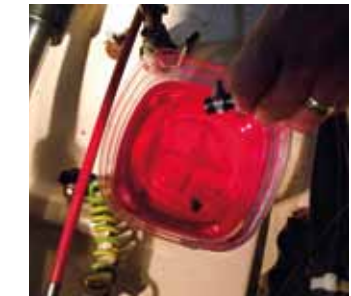
A clogged fuel tank pick-up led to problems further down the supply line at the primary filter
