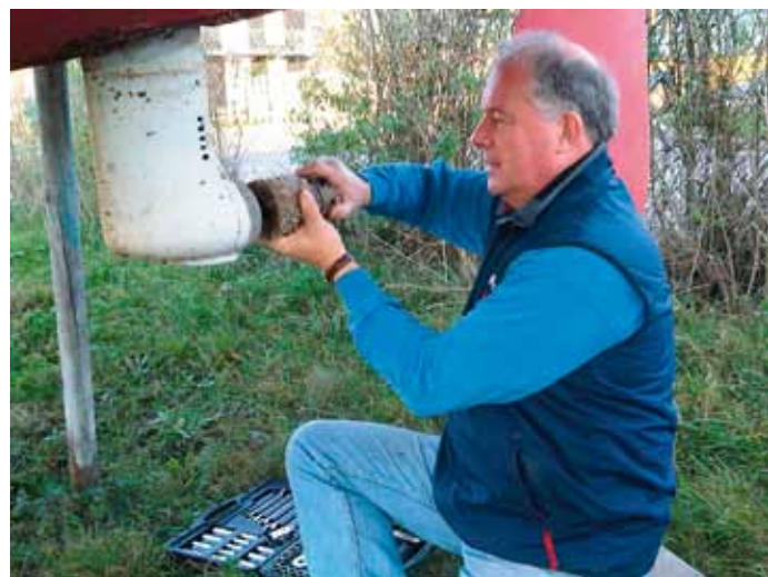
Barnacles cover the prop, and the saildrive may have to come out again
