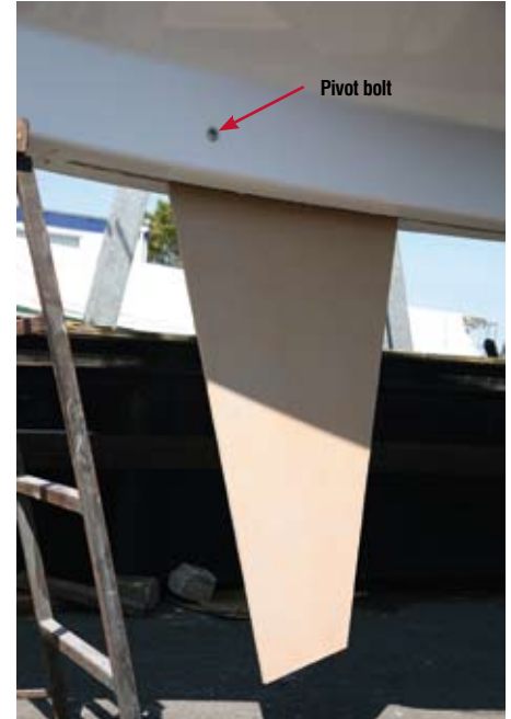
Before the centreplate is machined in mild steel, a template is made in MDF to ensure it fits the case in both raised and lowered positions
