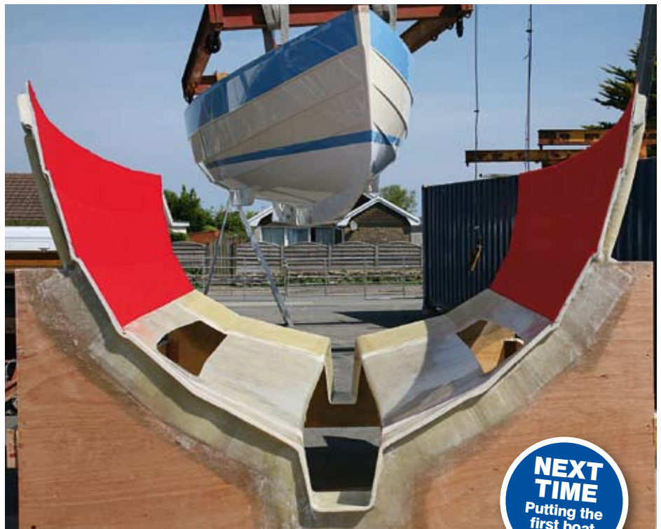
The 'ballast dolly', its shape taken from the hull plug, will support the hull while the ballast, bulkheads and interior moulding are fitted
