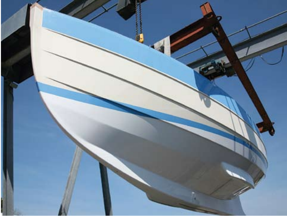
Released at last: the hull is lifted clear of the mould and its lines can be admired for the first time. Note the curved bilge stubs. A rubbing strake will sit immediately above the top chine
