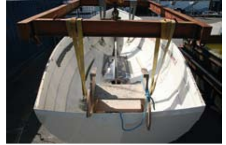
Bits of the interior plug still remain in the hull, principally around the centreplate case. The lifting points are bonded temporarily to the inside
