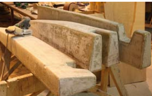
The plugs are made into fully enclosed boxes and smoothed and sanded, ready to be painted and delivered to the foundry
