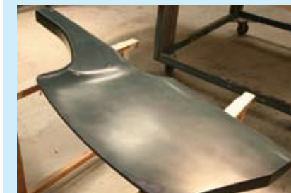
A plug is made for the transom-hung rudder
