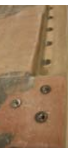
Hardware is bolted through the deck: a stanchion base in the foreground, and the track for the yankee
