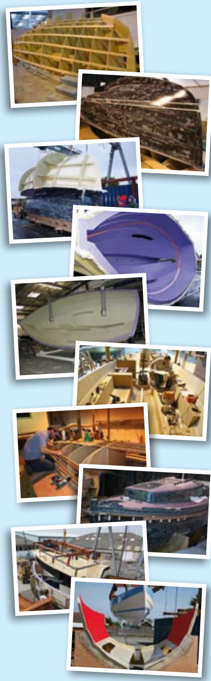
A WEIGHTING GAME The sections of balsa and plywood that will be laminated into the deck moulding are weighed down. Plywood is used where hardware is to be fitted; elsewhere it's balsa
