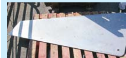
The centreplate arrives. Made from 20mm galvanised steel, it weighs 140kg (309lb)
