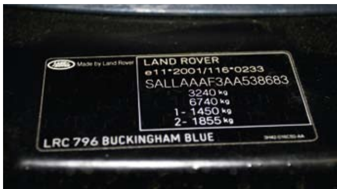
Weight figures will be on a stamped plate or sticker somewhere on your vehicle, usually under the bonnet or inside a door frame. In this example on the Land Rover Discovery 4, the Maximum Authorised Mass (MAM) is 3,240kg and the Maximum Combination Weight (MCW) is 6,740kg
