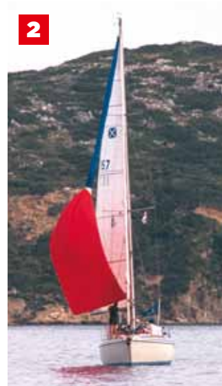
2 With the halyard and tack strop secured, partially unshathe the sail and secure the sock's control line before taking up the slack and securing the working sheet
