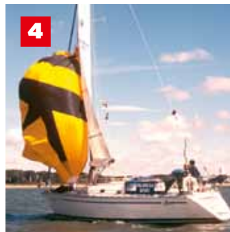
It's then just a matter of hauling down the sock until the sail is completely re-sheathed and secured
