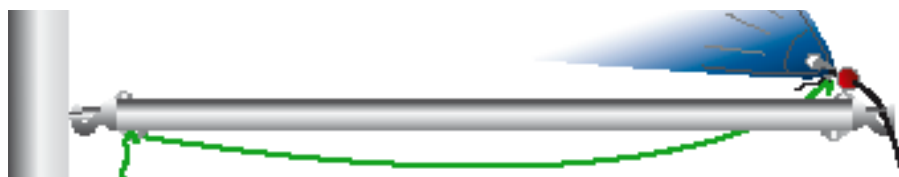
The emergency cord is tied between the snap shackle on the chute's tack and the pole's inboard end
