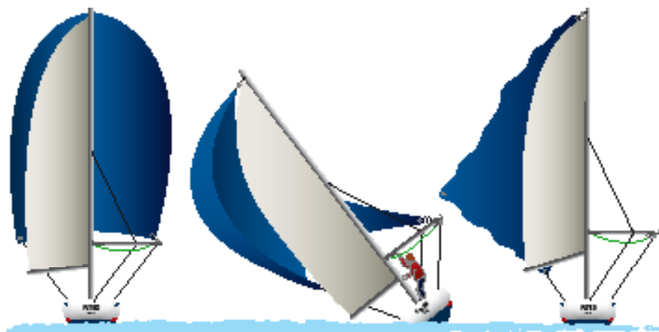
If the wind picks up unexpectedly, trip the line with one pull from a position near the mast
