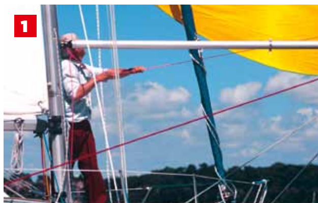
LEFT: With the boat on a broad reach, a single sharp pull on the cord, from a stable position near the mast, trips the tack of the chute
