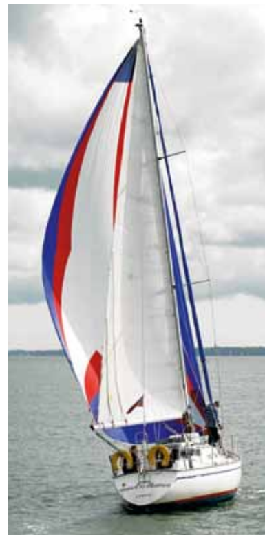
On the wind, tighten the halyard and tack strop for a straight leading edge
