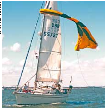
If the wind picks up unexpectedly, trip the line with one pull from a position near the mast
