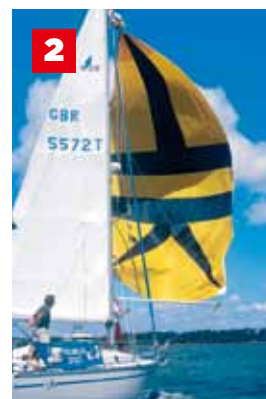
RIGHT: With the chute's tack disconnected from the pole, the sail loses power instantly
