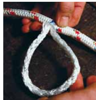
Braid-on-braid has a braided core as well as a cover. The core is much more softly laid than the outer sheath
