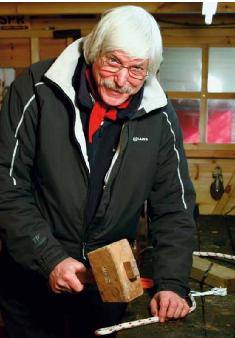
Tom Cunliffe uses a mallet to help the rope's core run smooth as he splices an eye into a length of braidline
