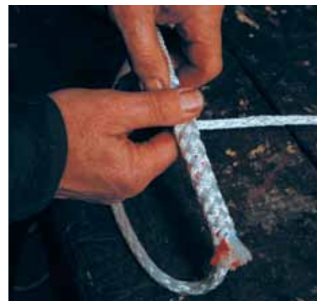
17 Then gingerly pull the coat back so that its end just disappears inside the core. →
