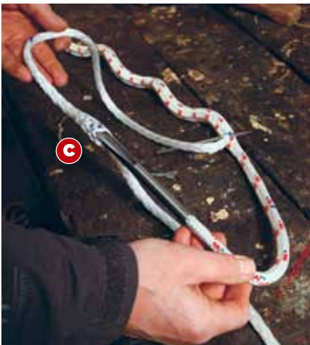
12 Open up the core at Mark C (the mark nearest the core's end), insert the fid.
