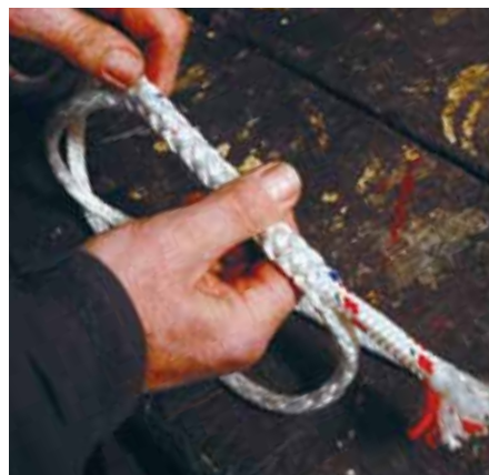
16 Next, very carefully, milk the core so that it closes neatly around the coat.
