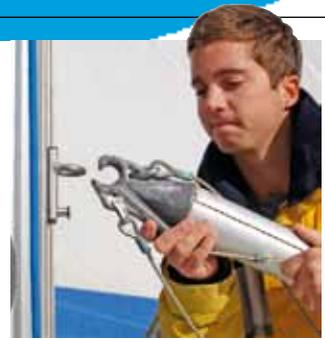
ABOVE: An 'end for end' pole has identical end fittings and jaws
