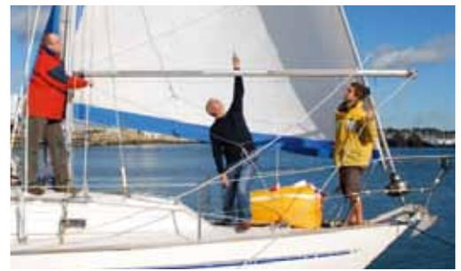
ABOVE: The topping lift is connected to an upper bridle and the downhaul connected to a lower bridle
