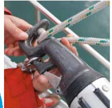
With the pole-end hanging just above the foredeck and with the new working guy in hand, the old working guy is unclipped. Then, taking care to feed it into the pole's jaws the correct way (as shown above), the new working guy is attached before the pole is raised and pulled back until it once again takes the load on the spinnaker. Slackening the new lazy sheet and guy then completes the gybe.
