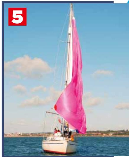
ABOVE: Haul smartly on the guy and ease the downhaul as the pole is pulled back. Be ready for the increased load as the spinnaker starts to fill as it's dragged out of the wind shadow
