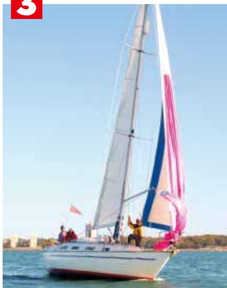
ABOVE: With the sheet secured and the guy around a winch ready to be hauled, hoist away on the spinnaker halyard as quickly as possible
