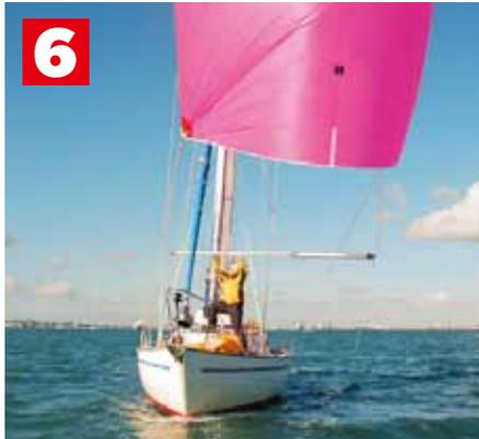
ABOVE: Swing the pole inboard again and unclip it from the old working guy. Then lead the end of the pole back towards the mast attachment. Stand by to readjust all of its control lines
