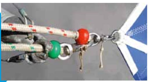
ABOVE: A swivel shackle prevents twists. A plastic ball prevents it jamming in the pole's jaw
