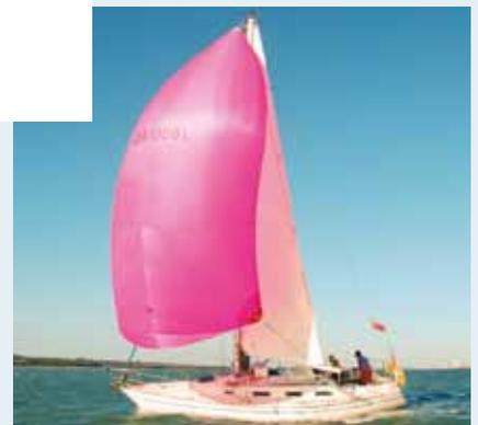
ABOVE: As the apparent (or true) wind rises, flatten the spinnaker to lower its centre of effort, reducing its tendency to roll the boat, by lowering the pole and moving the sheet-lead slightly forward
