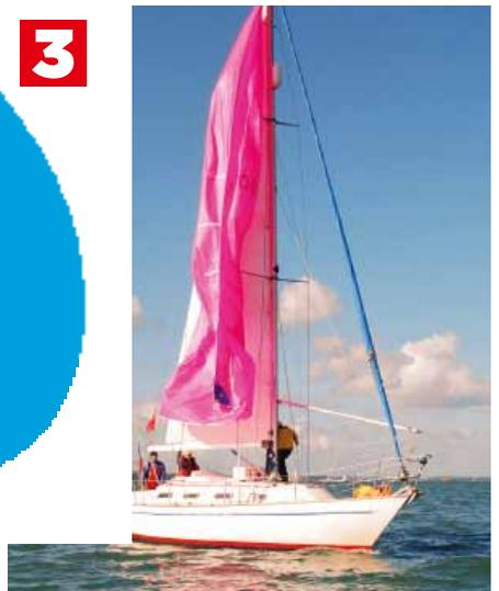
*ABOVE: Haul in on the sheet while the spinnaker flags downwind in the lee of the mainsail*
