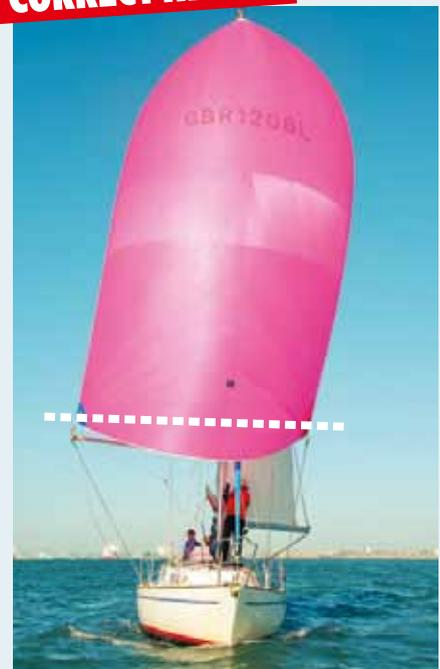
ABOVE: With the pole at the right height (tack and clew level) the spinnaker pulls evenly and helps keep the boat upright in a lively seaway
