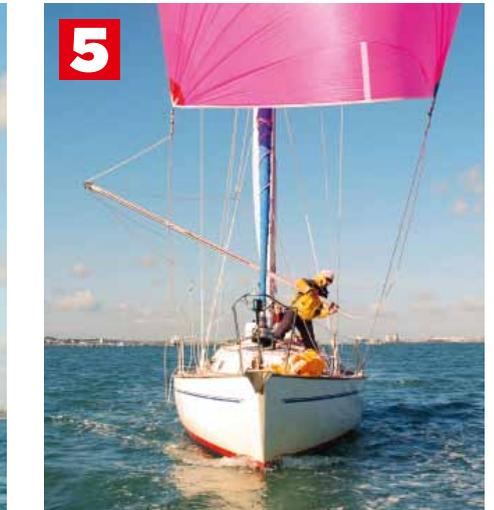
ABOVE: Clip the end of the pole onto the new working guy. Note that at this stage both guys are still attached to the ends of the pole
