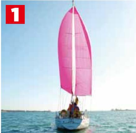
ABOVE: On a dead run, haul the mainsail in flat to funnel the wind evenly. Take the load of the spinnaker onto both sheets, then ease the guy, topping lift and downhaul to create some working slack for the pole
