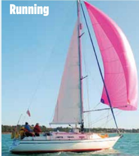
ABOVE: Before turning from a run onto a reach, be aware of the tendency for the pole to rise (and potentially induce a broach) if the guy and downhaul aren't kept under constant tension
