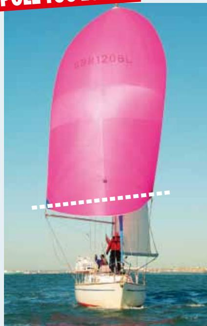
ABOVE: If the pole is too low (the tack lower than the clew), the sail will have a tendency to swing and roll the boat to windward
