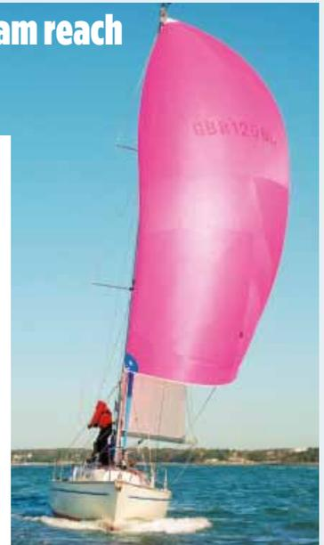
ABOVE: Coming onto a beam reach, ease the guy and keep tensioning the downhaul until the pole is braced just off the forestay
