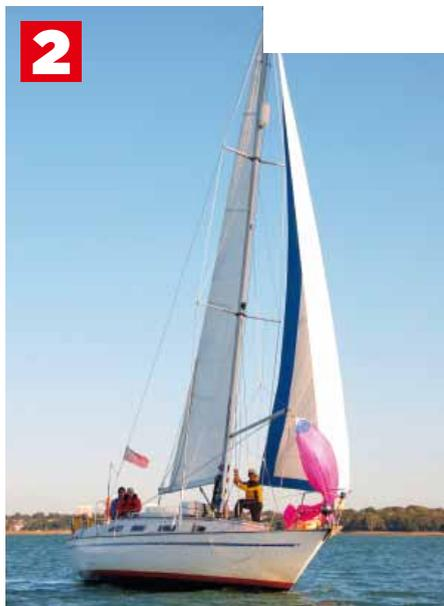
ABOVE: Take the slack out of the sheet, then tension the guy until the tack is pulled to the pole-end and the pole is just off the forestay
