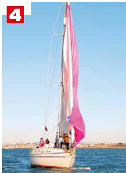
ABOVE: Keep hoisting the spinnaker quickly (there should be very little load at this stage) until it's all the way up, then secure its halyard
