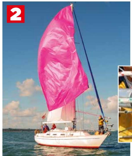
*ABOVE AND INSET: Trip the tack with a sharp pull on the sheet's snap shackle trip-cord*
