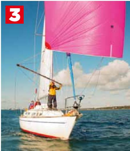
ABOVE: With the pole clipped around the old working guy and hanging from its topping lift, swing it across the boat towards the new one
