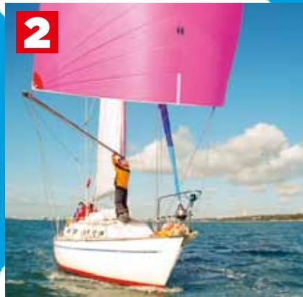
ABOVE: With the load on both sheets and as the boat tracks dead downwind, carefully unclip the pole from the mast. Leave the jaws at the outer end of the pole clipped around the old working guy
