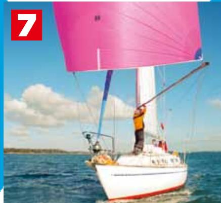
ABOVE: With the pole back on the mast and slack taken out of the topping lift and downhaul, take the load on the new working guy and sheet. Ease the mainsail to starboard, slacken the lazy sheet and complete the gybe
