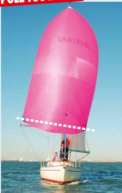
ABOVE: If the pole is too high (the tack higher than the clew) the sail will tend to swing and roll the boat to leeward in a stronger wind
